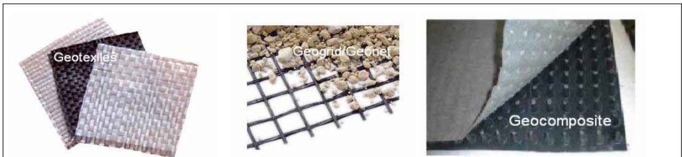
Figure 9: Photographs of various types of geosynthetics. From left to right: woven geotextiles, geogrid, and geocomposite.
