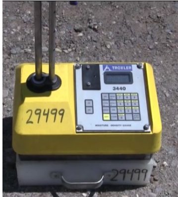
Standardizing the nuclear density gauge
