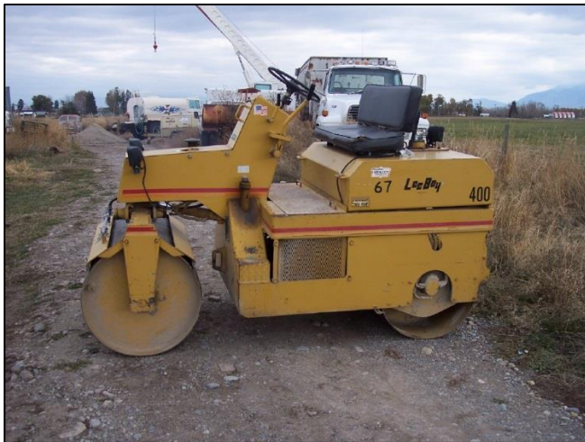
Photographs 7 and 8: Dual drummed steel vibratory roller and rubber-tired pneumatic roller.
